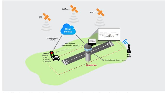
DRIWS is based on satellite navigation and wireless communication between the vehicle and air traffic control.
